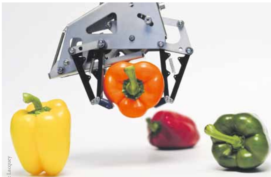
An industrial gripper developed by a private company, elaborating on a prototype developed at TU Delft.
